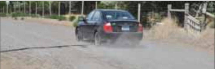
A vehicle travels a rotomilled portion of Johnstone Road, showing how a roadway treated with a sugar beet byproduct (above) reduces dust compared to untreated (left).
