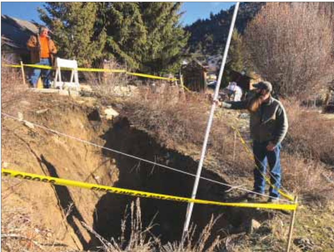
BLM Idaho Abandoned Mines team leader Phil Barbarick (left) and BLM heavy equipment operator Adam R. Nelson take measurements of the collapsed mineshaft. BLM photo
