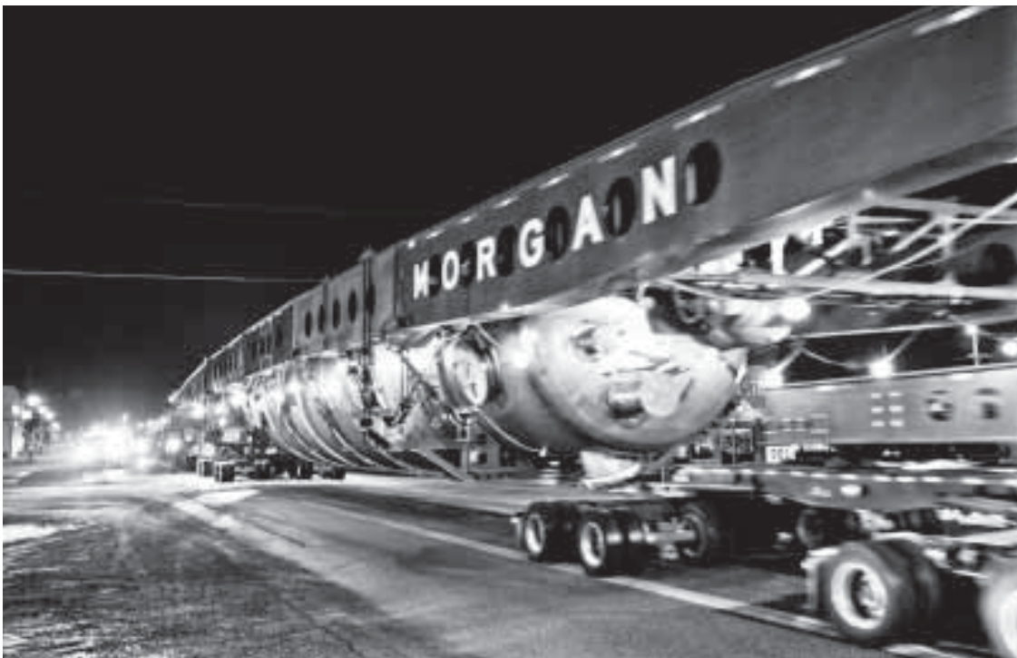
The tires supporting the first of three megaload shipments of oil refinery equipment hug the fog line in the first block of East Idaho Avenue as support vehicles, including pilot vehicles and Idaho State Police troopers, tail the 376-foot-long cargo. The 450-ton water purification unit was hauled from Vale, Ore., to the old port of entry outside of Marsing overnight Sunday, arriving in Homedale at midnight and reaching its destination two hours later. The trucks and trailer will remain outside Marsing for Christmas because the Idaho Transportation Department permit won't allow travel again until 10 p.m. on Thursday.
