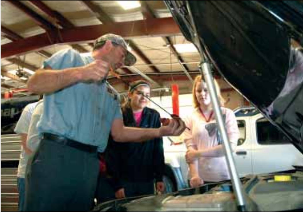
Jason Conant, mechanic for Matteson's repair shop in Homedale, shows Girl Scouts Maya Correa, left, and Megan Aman how to check the oil levels in a car.
