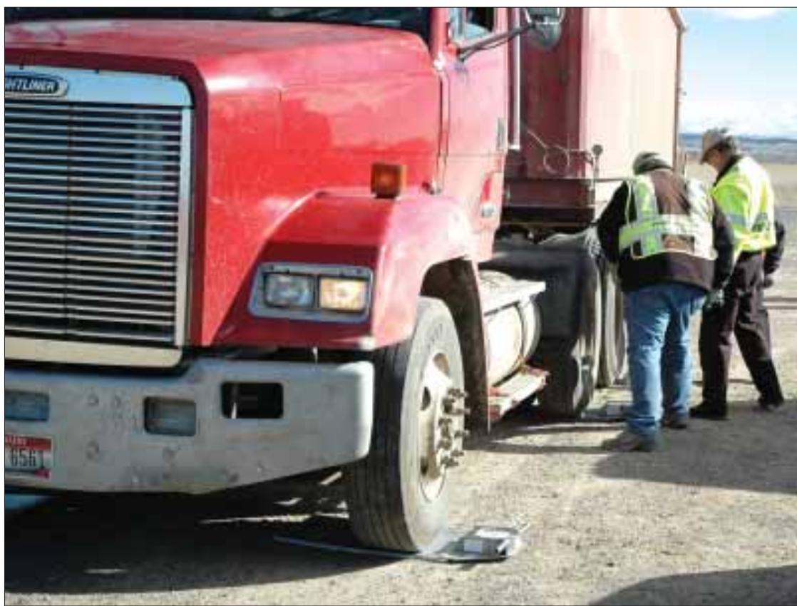
Above: Idaho State Police trooper Seth Uhlenkott checks a silage truck's braking system as a Port of Entry employee examines another part of the rear axle. Below: Port of Entry inspectors weigh a semi at a roving scales site on Johnstone Road.
