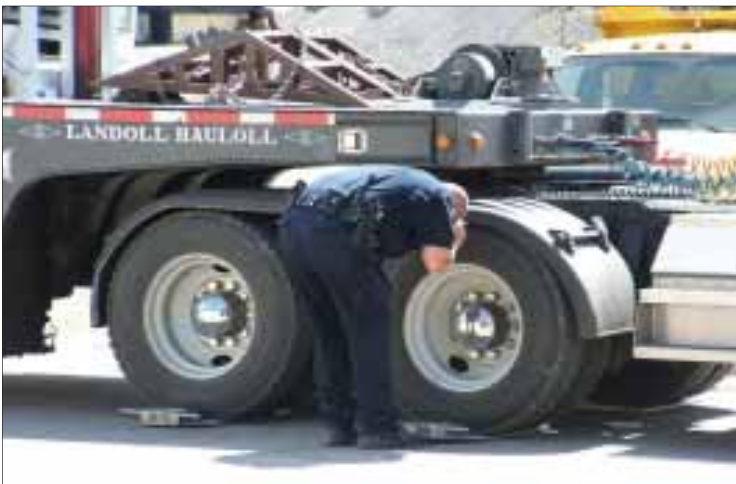
Above: A law enforcement official inspects the brakes of a semi at an Idaho Transportation checkpoint in Idaho City. Left: Boise County sheriff's deputies inspect a truck at an Idaho Transportation Department checkpoint in Idaho City. Photos courtesy ITD
