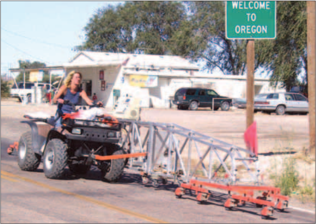
Highway 19 road work A worker from the Idaho Department of Transportation drives a Profilograph to measure grooves and bumps on Highway 19 last week in preparation of a two-week project.
